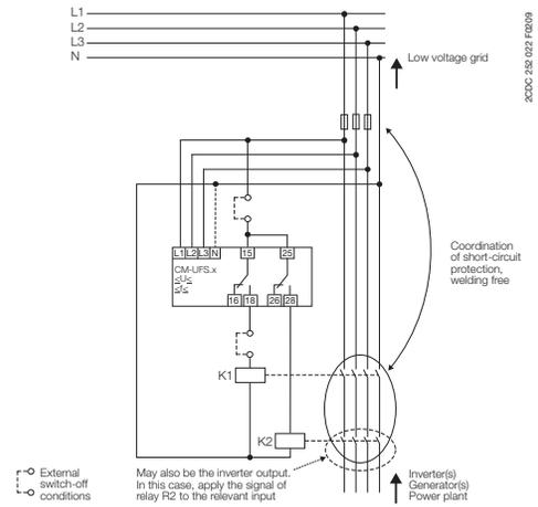
**Automatized grid connection instead of a permanently accessible switching point with a disconnection function**
