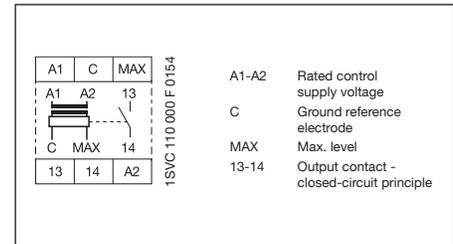
If a metal tank is used, the ground reference electrode C is not required. In this case the cable can be connected directly to the metal surface of the tank.
