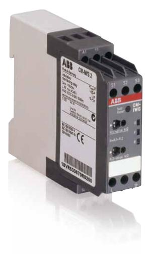
The CM-IWS.2 is used to monitor insulation resistance in accordance with IEC 61557-8 in pure IT AC systems. Measured are insulation resistances between system lines and system earth. When falling below the adjustable threshold values, the output relays switch into the fault state.
