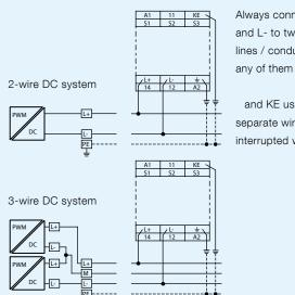
Always connect L+ and L- to two different lines / conductors,
