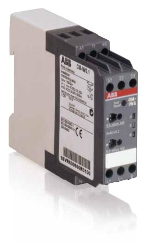
The CM-IWS.1 and CM-IWN.1 serve to monitor insulation resistance in accordance with IEC 61557-8 in unearthed IT AC or DC systems. Measured are insulation resistances between system lines and system earth. When falling below the adjustable threshold values, the output relays switch into the fault state. With CM-IWS.1 und CM-IWN.1 a pulsating measuring signal is fed into the system to be monitored and the insulation resistance calculated.
