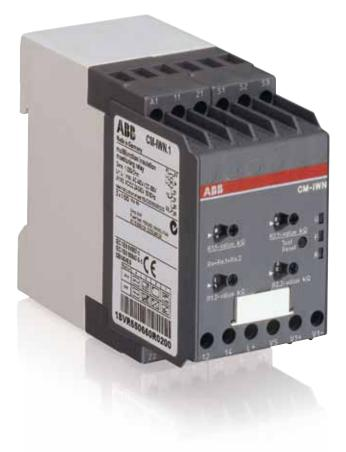
The pulsating measuring signal from CM-IWS.1 and CM-IWN.1 alters its form in dependence of the insulation resistance and the system leakage capacitance. From this altered form the change in the insulation resistance is forecast.
