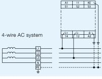
Always connect L+ and L- to two different lines / conductors, any of them
