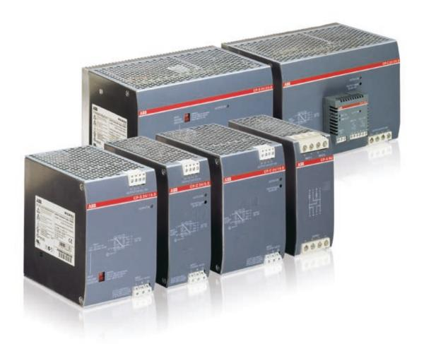
The power supply units in the CP-S and CP-C range are ABB's high-end solutions. Designed with an integrated 50 % power reserve and an efficiency of approximately 89 % these are the perfect products for all complex, highly reliable applications. All the devices cover the U-I output characteristic and are built with thermal protection which switches off in case of overheating.
