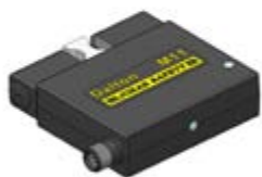
Dalton M11 with 8-pin male contact
