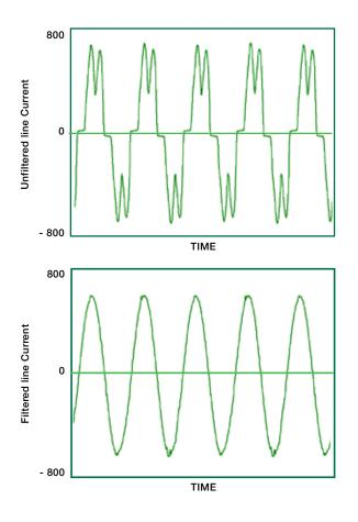
The closed loop control concept also enables the filter to demonstrate excellent performance for achieving target power factor and load balancing.
