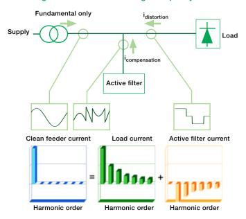
An ABB PQF active filter is a power electronics based electrical equipment that is installed parallel to the polluting loads. It monitors the line current harmonics, as well as the customer requirements programmed by the user. It can then generate for each harmonic frequency a compensation current in perfect phase opposition to the polluting current.
