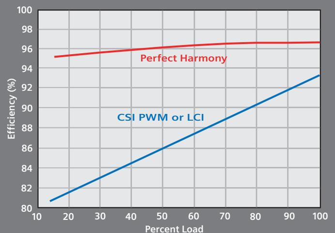
System efficiency includes isolation transformer, harmonic filter, power factor correction and drive.
