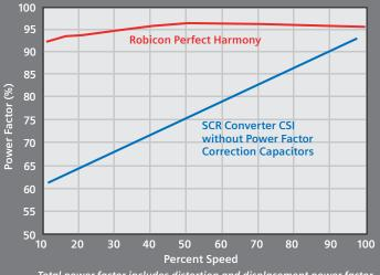
Total power factor includes distortion and displacement power factor.
