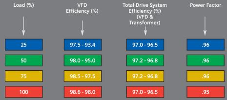
Efficiency and power factor values are based on centrifugal load characteristics for torque and speed.
