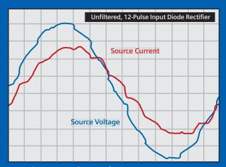
12-Pulse Harmonic Waveform 5.9% total voltage distortion 8.8% total current distortion
