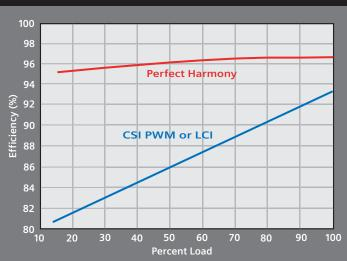
System efficiency includes isolation transformer, harmonic filter, power factor correction and drive.
