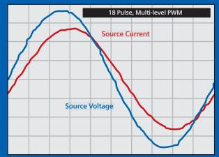
**Perfect Harmony Series Waveform** less than 3% total voltage distortion less than 5% total current distortion Meets IEEE 519-1992 at the input to the isolation transformer
