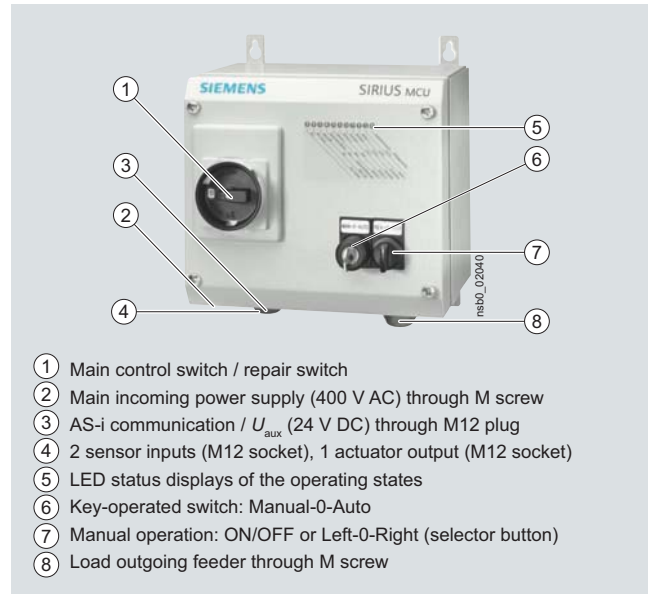
MCU for AS-i, metal enclosure, electromechanical switching
