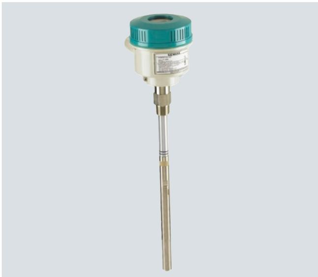
Pointek CLS300 (digital version) is an inverse frequency shift capacitance level switch with optional rod/cable choices and configurable output. It is ideal for detecting liquids, solids, slurries, foam and interfaces in demanding conditions where high pressure and temperatures are present. The digital version includes PROFIBUS PA, an LCD display, and advanced diagnostic features.
