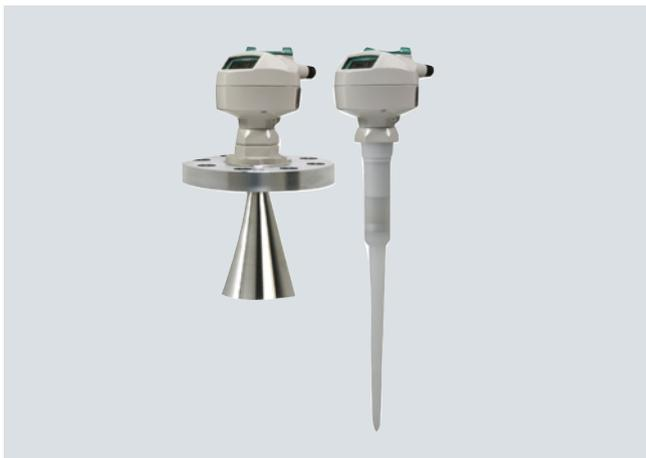
SITRANS LR200 is a 2-wire, 6 GHz pulse radar level transmitter for continuous monitoring of liquids and slurries in storage and process vessels including high temperature and pressure, to a range of 20 m (66 ft).
