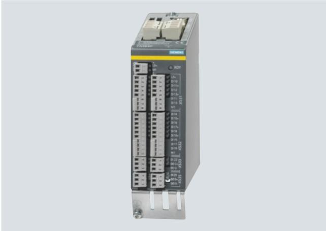
The TM54F Terminal Module is a dual-processor I/O interface with 4 fail-safe digital outputs and 10 fail-safe digital inputs for utilization of the Safety Integrated functions of the SINAMICS S120 drive system over external actuators and sensors.
