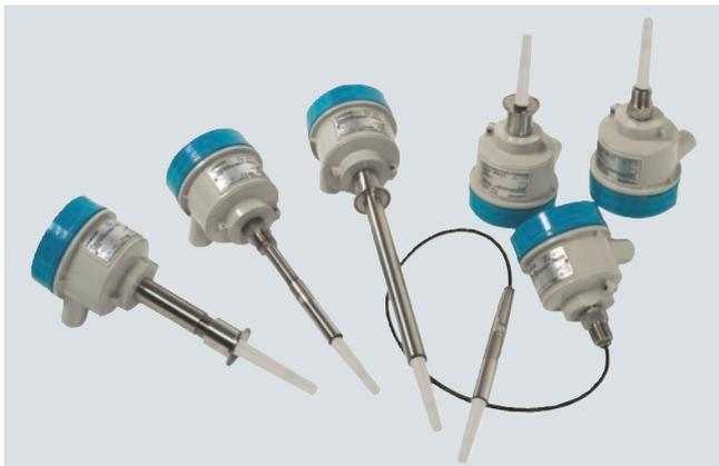
Pointek CLS200 (digital version) is a versatile inverse frequency shift capacitance level switch with optional rod/cable choices and configurable output, ideal for detection of liquids, solids, slurries, foam and interfaces. The digital version includes PROFIBUS PA, an LCD display, and advanced diagnostic features.
