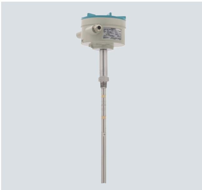
Pointek CLS 500 is an inverse frequency shift capacitance level switch for detecting interfaces, solids, liquids, toxic and aggressive chemicals in critical conditions of high temperature and pressure.
