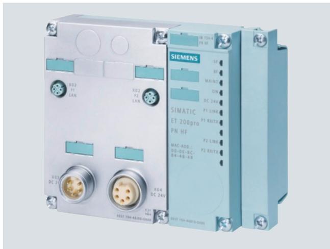
Interface module for processing the communication between ET 200pro and a higher-level controller over PROFINET IO.
