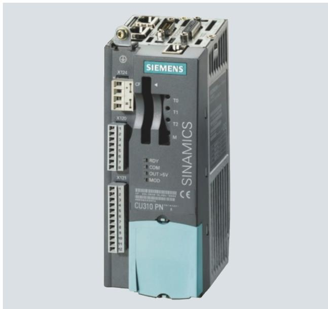
The CU310 PN Control Unit is designed for the communication and open-loop/closed-loop control functions of a Power Module. The CU310 PN combined with a Power Module and CompactFlash Card creates a powerful single-axis AC drive. The communication link to the higher-level control is provided by PROFINET IO.
