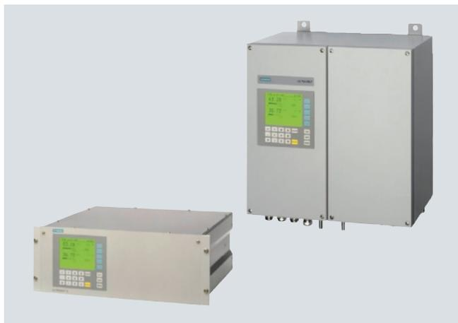
The ULTRAMAT 6 single-channel or dual-channel gas analyzers operate according to the NDIR two-beam alternating light principle and measure gases highly selectively whose absorption bands lie in the infrared wavelength range from 2 to 9  $\mu\text{m}$ , such as CO, CO<sub>2</sub>, NO, SO<sub>2</sub>, NH<sub>3</sub>, H<sub>2</sub>O, CH<sub>4</sub> and other hydrocarbons.
