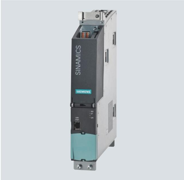
The communication, open-loop and closed-loop control functions for one or more Motor Modules and the Line Module are executed in a CU320-2 DP Control Unit. The CU320-2 DP Control Unit is designed for multi-axis operation.
