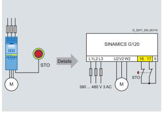
Integrated safety via fail-safe inputs
