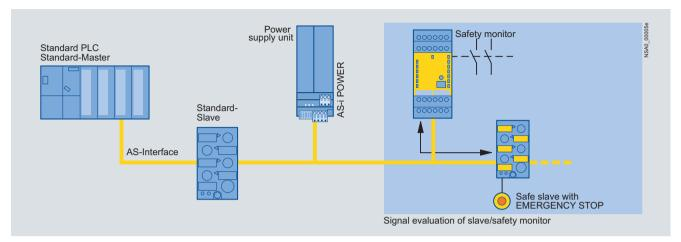
Secure communication and standard communication on AS-Interface
