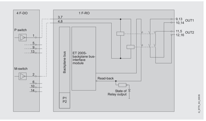
The block diagram shows the control via 4F-DO 24 V DC/2A PROFIsafe (6ES7138-4FB02-0AB0). The control circuit must be routed to the terminals 3, 4 or 7, 8. One channel of the F-DO can also be used for control of multiple F-RO modules (group shutdown).
