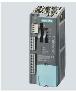
The CU310 PN Control Unit is designed for the communication and open-loop/closed-loop control functions of a Power Module. The CU310 PN combined with a Power Module and Compact-Flash Card creates a powerful single-axis AC drive. The communication link to the higher-level control is provided by PROFINET IO.
