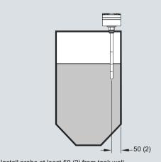
Install probe at least 50 (2) from tank wall.
