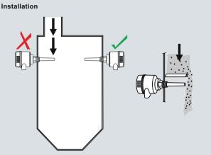
Keep unit out of path of falling material, or protect probe from falling material.
