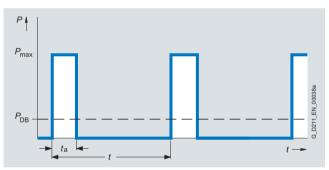
Load diagram for Braking Module in Blocksize format
