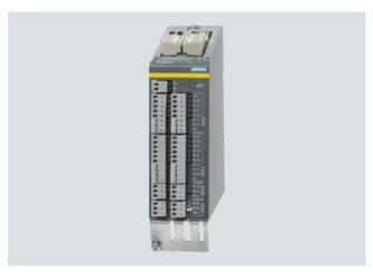
The TM54F Terminal Module is a dual-processor I/O interface with 4 fail-safe digital outputs and 10 fail-safe digital inputs for utilization of the Safety Integrated functions of the SINAMICS S120 drive system over external actuators and sensors.
