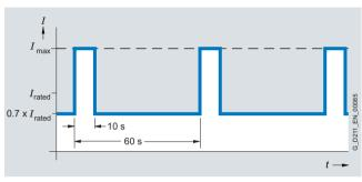
S6 duty cycle with initial load with a duty cycle duration of 60 s
