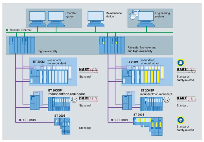
Common engineering system for basic process control system and safety instrumented system
