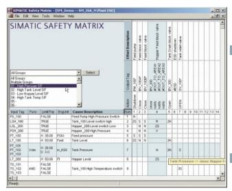
The SIMATIC Safety Matrix which can be used in addition to the CFC is an innovative safety lifecycle tool from Siemens that can be used not only for user-friendly configuration of safety applications, but also for their operation and service. The tool, which is based on the proven principle of a cause & effect matrix, is ideally suited to processes where defined statuses require specific safety reactions.
