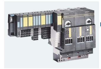
The Fail-safe motor starter has been developed on the basis of the High-Feature motor starter. It differs in that, in addition to a motor starter protector and contactor assembly, a safe solid-state evaluation circuit is installed for error detection purposes which makes the motor starter fail-safe.
