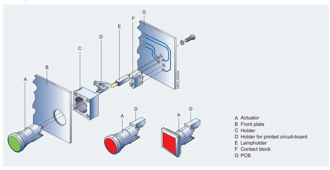
Contact blocks for use on printed circuit boards.
