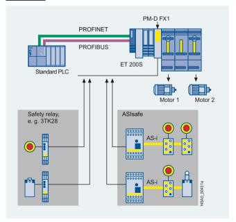
ET 200S safety motor starter Solutions local with 2 external safety assemblies (= safety relays or ASIsafe monitors) and with fail-safe motor starters (PM-DFX1 application).
