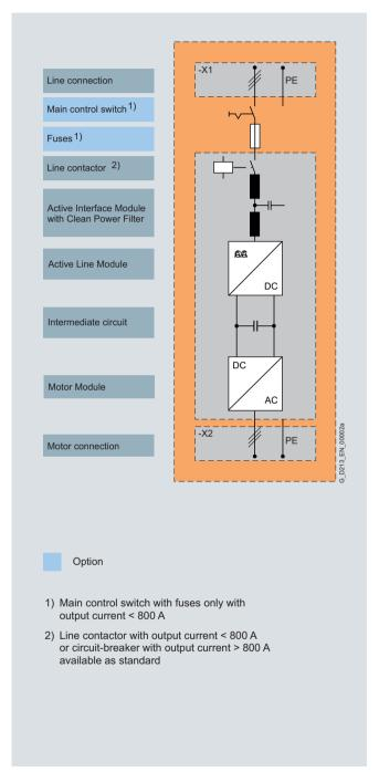
Basic design of a SINAMICS S150 drive converter cabinet unit with a number of version-specific options
