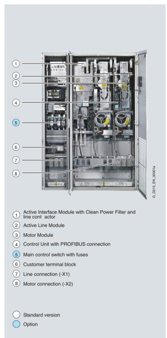
Example of the design of a SINAMICS S150 drive converter cabinet unit
