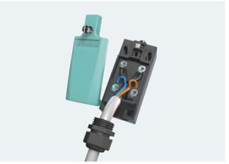
These position switches can be wired quickly and easily as an added customer benefit. The connecting cable is first connected to the terminals of the contact block and then guided through a slit into the cable gland opening. The time saved through this new connection method is approx. 20 to 25 %.
