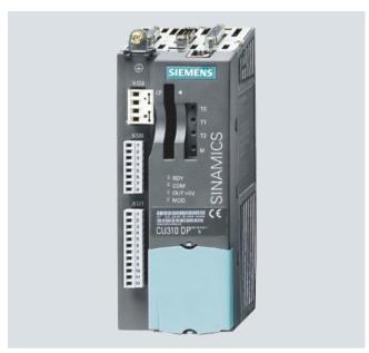
The CU310 DP Control Unit provides the communications and open-loop/closed-loop control functions for a Power Module. The CU310 DP combined with a Power Module and Compact-Flash Card creates a powerful single-axis AC drive with a PROFIBUS interface to a higher-level control.
