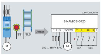
Integrated safety via fail-safe inputs
