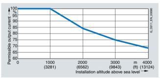
Output current as a function of installation altitude
