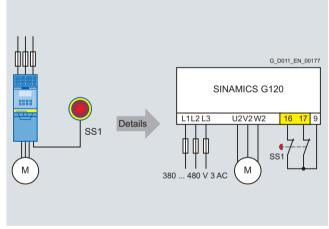
Integrated safety via fail-safe inputs
