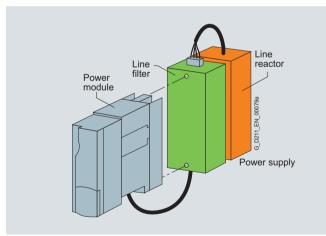
PM340 in frame size FSA with line reactor and line filter
