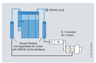
Example of a dual-encoder system on a spindle
