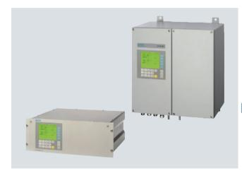
The ULTRAMAT 6 single-channel or dual-channel gas analyzers operate according to the NDIR two-beam alternating light principle and measure gases highly selectively whose absorption bands lie in the infrared wavelength range from 2 to 9  $\mu m$ , such as CO, CO<sub>2</sub>, NO, SO<sub>2</sub>, NH<sub>3</sub>, H<sub>2</sub>O, CH<sub>4</sub> and other hydrocarbons.
