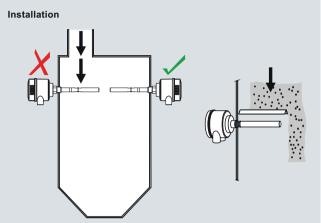
Keep unit out of path of falling material, or protect probe from falling material.
