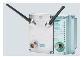
Interface module for handling communication between ET 200pro and host PROFINET IO controllers over Industrial Wireless LAN (IWLAN) radio networks for 2.4 GHz or 5 GHz with data transfer rates up to 54 Mbit/s.
