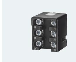
The three-pole contact block with snap-action or slow-action contacts is regularly available for all enclosure forms. The same installation space is required as for a two-pole block. The version with 1 NO + 2 NC offers for example more safety through redundant shutdowns (2 NC contacts) with simultaneous signaling (1 NO contact). The three-pole blocks are also available with make-before-break and with 2 NO + 1 NC.
