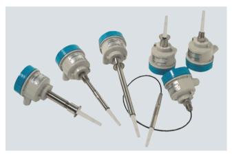
Pointek CLS200 (digital version) is a versatile inverse frequency shift capacitance level switch with optional rod/cable choices and configurable output, ideal for detection of liquids, solids, slurries, foam and interfaces. The digital version includes PRO-FIBUS PA, an LCD display, and advanced diagnostic features.
