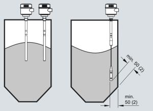
Install probe at least 50 mm (2") from tank wall. Note angle of repose and adjust accordingly.
