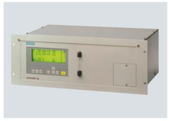
The ULTRAMAT 23 gas analyzer can measure up to 4 gas components at once: A maximum of three infrared sensitive gases such as CO, CO<sub>2</sub>, NO, SO<sub>2</sub>, CH<sub>4</sub> plus O<sub>2</sub> with an electrochemical oxygen measuring cell.
