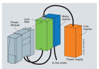
For configurations involving more than two base-type system components, e.g. line reactor + motor reactor + braking resistor, individual components must be mounted to the side of the PM340. In this instance, the line and motor reactors must be installed behind the PM340 and the braking resistor to the side.
