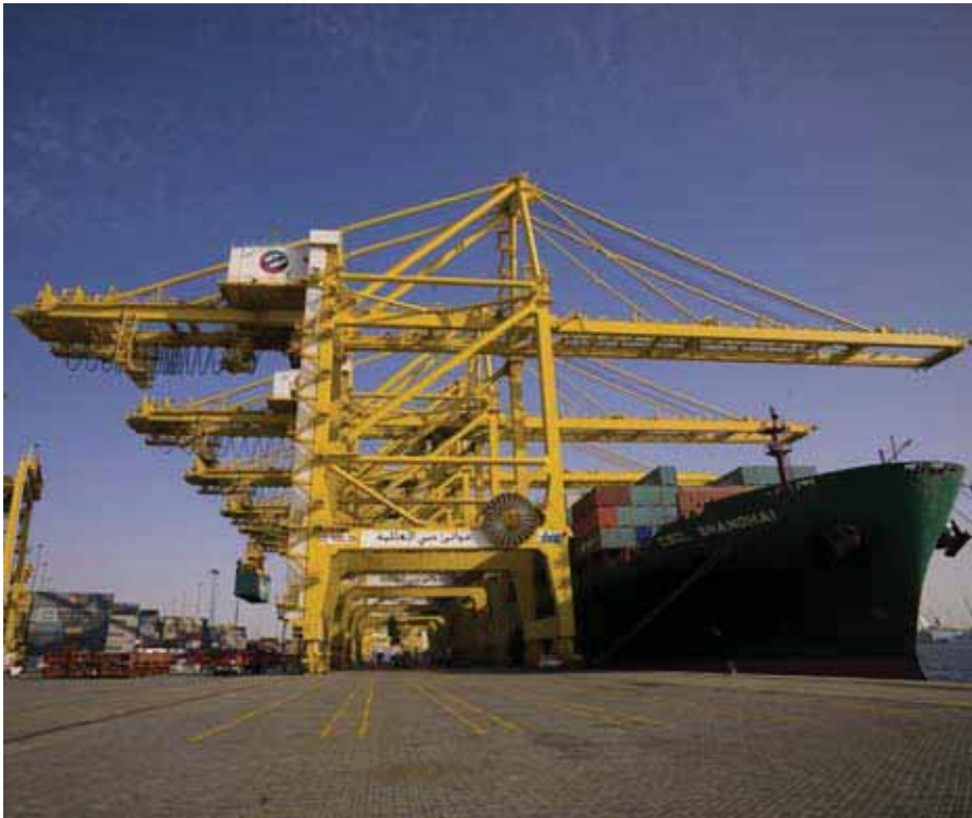
Example: STS crane, lifting capacity up to 120 t, trolley speed up to 250 m/min
