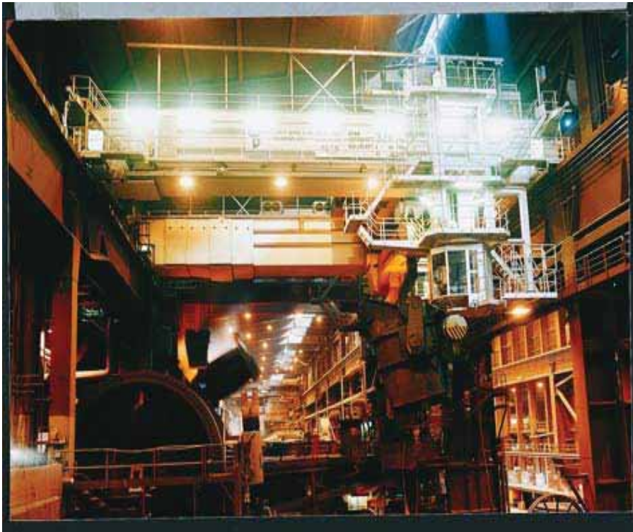
Example: Ladle crane, hoisting capacity 200 - 500 t, gantry speed approx. 60 m/min
