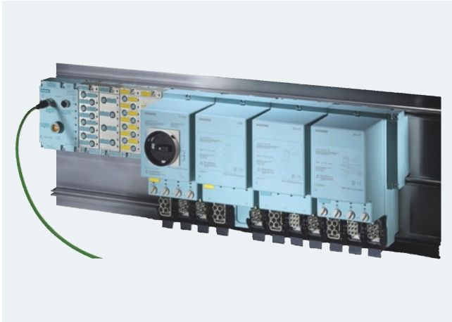
ET 200pro motor starter: Safety local isolator module, disconnecting module, Standard starter and High-Feature starter mounted on a wide module rack
