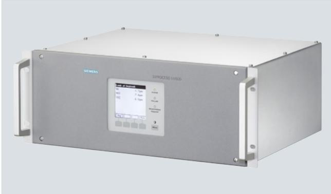
The function of the SIPROCESS UV600 gas analyzer is based on UV resonance absorption spectrometry. It also is used to measure very low NO, NO<sub>2</sub>, SO<sub>2</sub> or H<sub>2</sub>S concentrations in gases.
