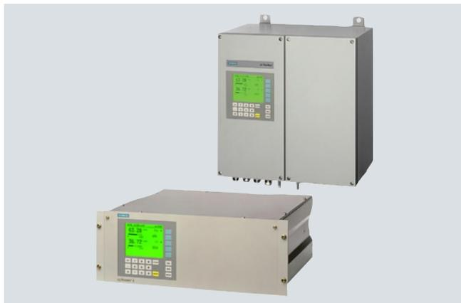
The ULTRAMAT 6 single-channel or dual-channel gas analyzers operate according to the NDIR two-beam alternating light principle and measure gases highly selectively whose absorption bands lie in the infrared wavelength range from 2 to 9  $\mu\text{m}$ , such as  $\text{CO}$ ,  $\text{CO}_2$ ,  $\text{NO}$ ,  $\text{SO}_2$ ,  $\text{NH}_3$ ,  $\text{H}_2\text{O}$  as well as  $\text{CH}_4$  and other hydrocarbons.
