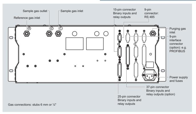
OXYMAT 6, 19" unit, gas and electrical connections
