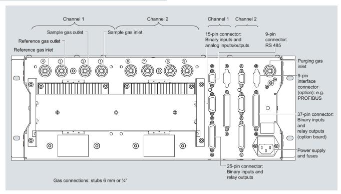
ULTRAMAT 6, 19" unit, gas and electrical connections (example: 2-channel version)
