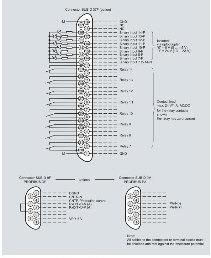
OXYMAT 6, 19" unit, pin assignment of AUTOCAL board and PROFIBUS connectors
