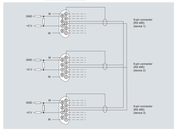
Bus cable with plug connections, example
