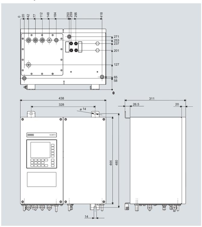
CALOMAT 62, field device, dimensions in mm
