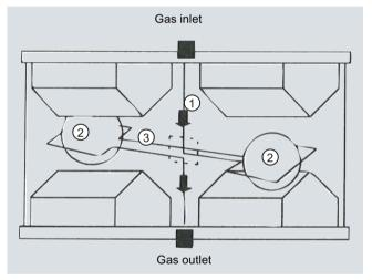
Operating principle of the paramagnetic oxygen cell
