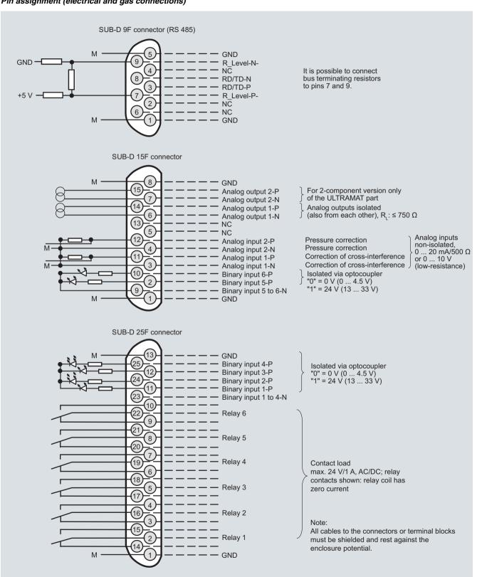
ULTRAMAT/OXYMAT 6, 19" unit, pin assignment
