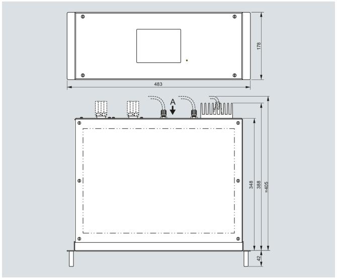
SIPROCESS UV600, 19" rack unit, dimensions in mm
