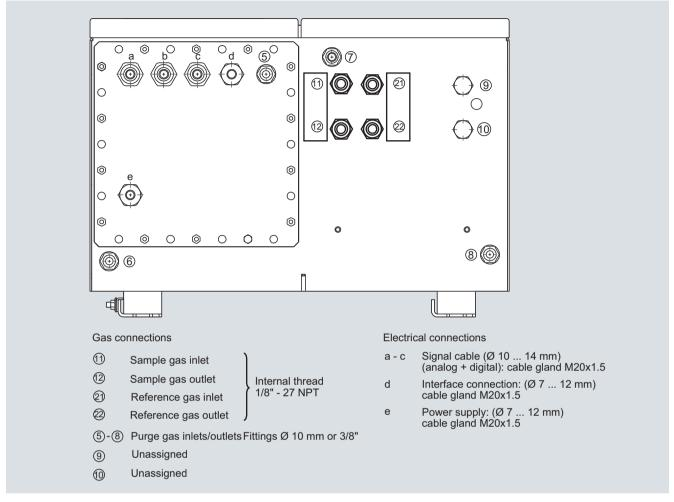
CALOMAT 62, field device, gas connections and electrical connections
