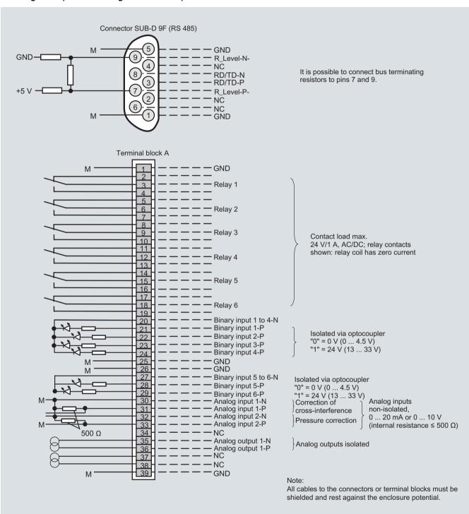
OXYMAT 6, field unit, connector and terminal assignment
