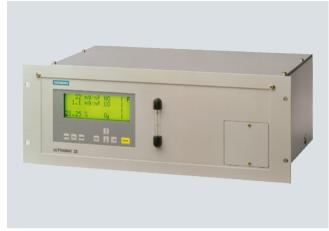
Up to four gas components can be measured simultaneously with the ULTRAMAT 23 gas analyzer: up to three infrared-active gases such as CO, CO<sub>2</sub>, NO, SO<sub>2</sub>, CH<sub>4</sub>, plus O<sub>2</sub> with an electrochemical oxygen sensor.
