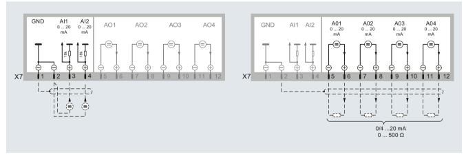
SIPROCESS UV600, pin assignment of the analog inputs X7 (Al1 and Al2) and analog outputs X7 (AO1 to AO4)
