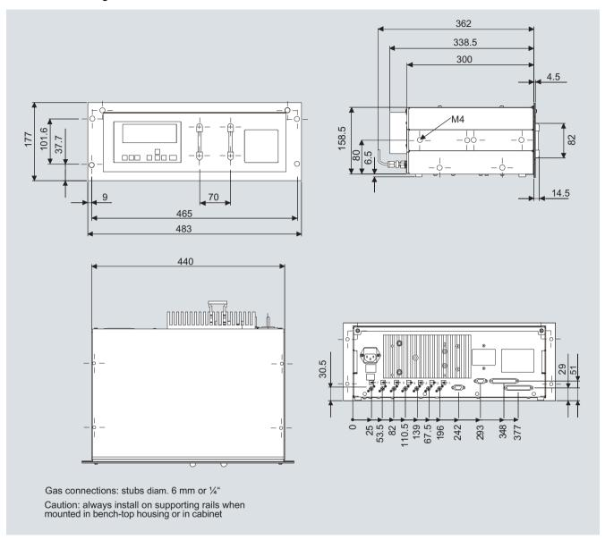
ULTRAMAT 23, 19" unit, dimensions in mm
