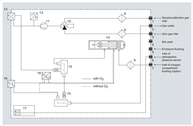
ULTRAMAT 23, 19" rack unit enclosure with internal sample gas pump and H<sub>2</sub>S sensor
