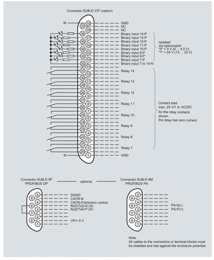
CALOMAT 62, 19" rack unit, pin assignment of the AUTOCAL board and PROFIBUS connectors
