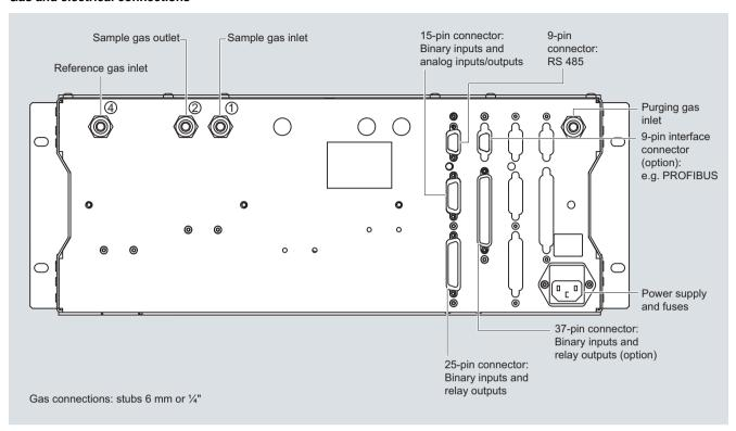
OXYMAT 61, 19" unit, gas and electrical connections
