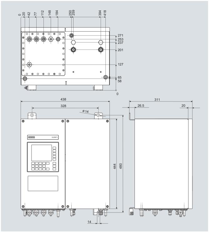
OXYMAT 6, field unit, dimensions in mm
