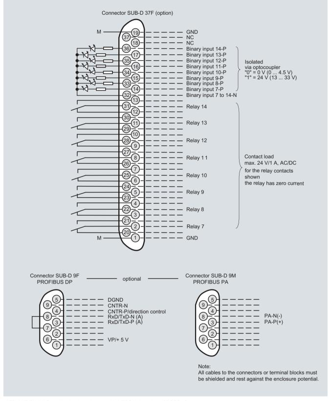
ULTRAMAT/OXYMAT 6, 19" unit, pin assignment of AUTOCAL board and PROFIBUS connectors
