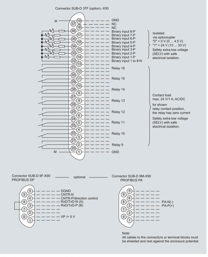
ULTRAMAT 23, pin assignment of the optional PROFIBUS interface board
