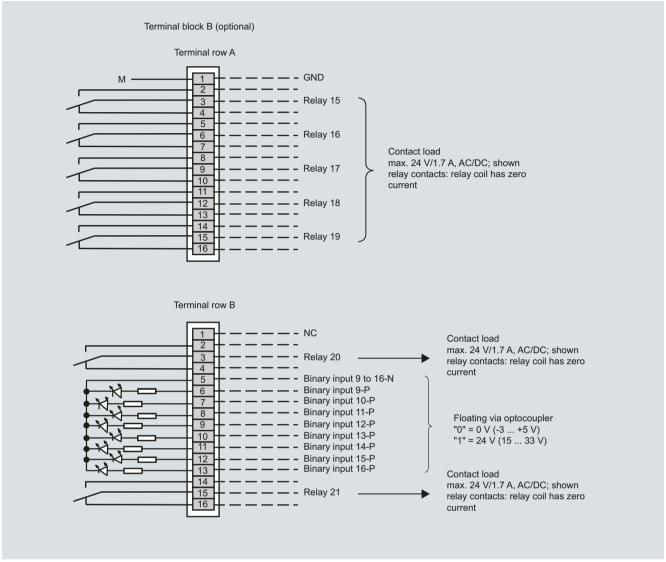
Terminal assignment, terminal block B, terminal rows A and B
