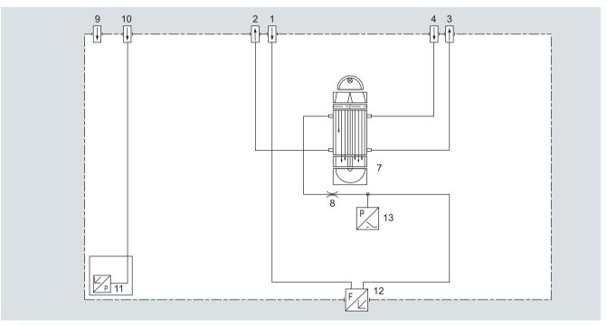
Gas path ULTRAMAT 6, single-channel unit, 19" unit, with flow-type reference cell (option)
