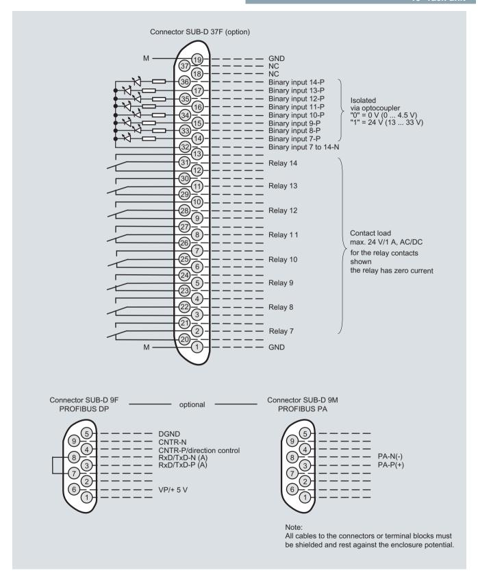
ULTRAMAT 6, 19" unit, pin assignment of AUTOCAL board and PROFIBUS connectors
