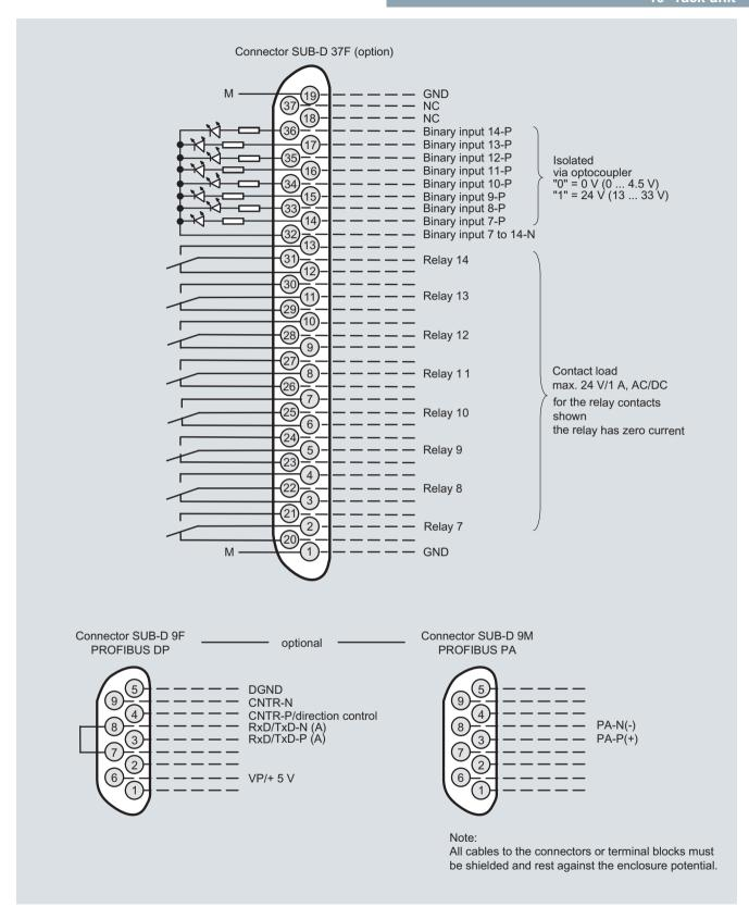
CALOMAT 6, 19" unit, pin assignment of AUTOCAL board and PROFIBUS connectors
