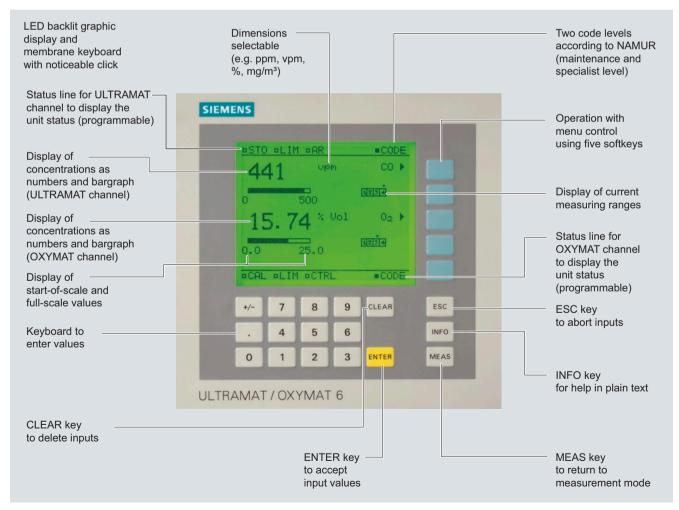
ULTRAMAT/OXYMAT 6, membrane keyboard and graphic display
