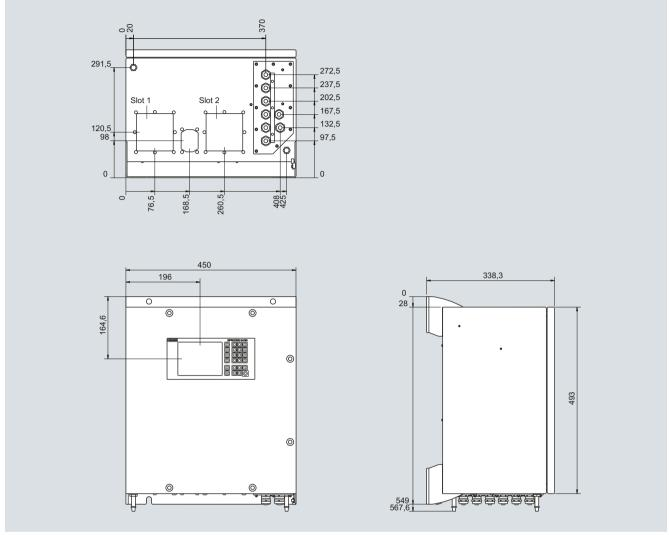
SIPROCESS GA700, wall housing, dimensions in mm
