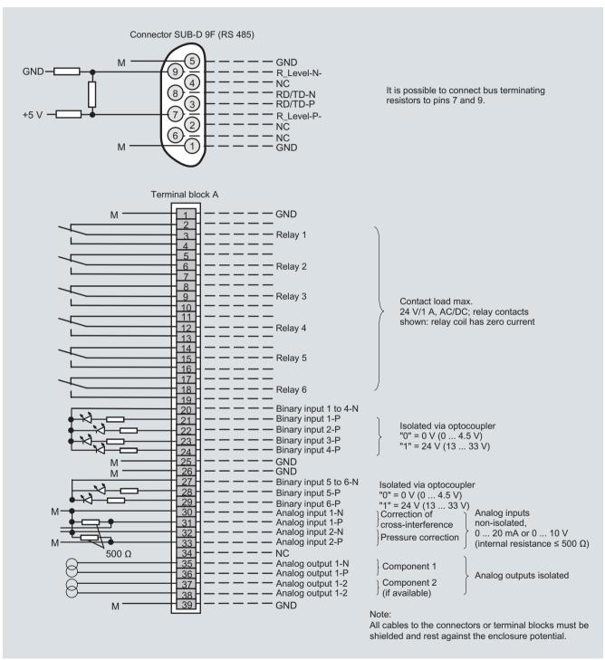
ULTRAMAT 6, field device, pin and terminal assignment
