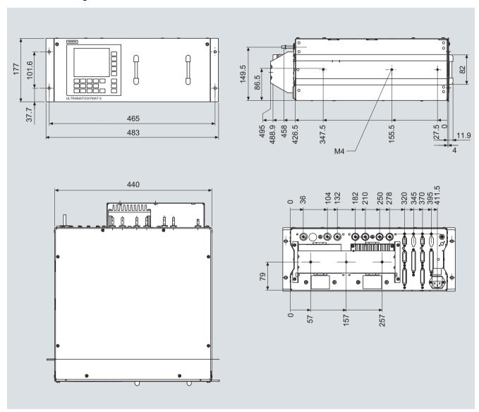
ULTRAMAT/OXYMAT 6, 19" unit, dimensions in mm
