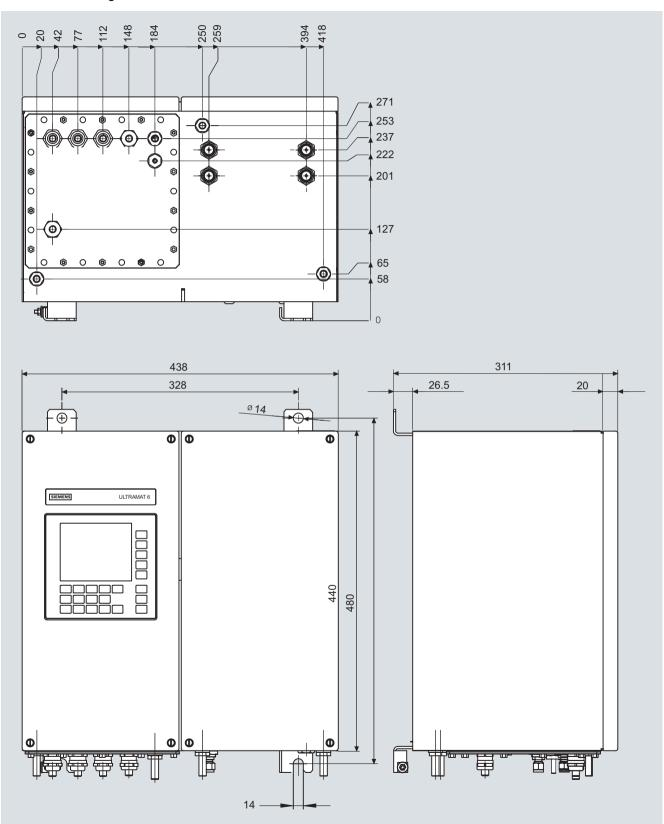
ULTRAMAT 6, field unit, dimensions in mm
