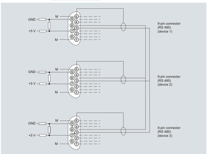
Bus cable with plug connections, example
