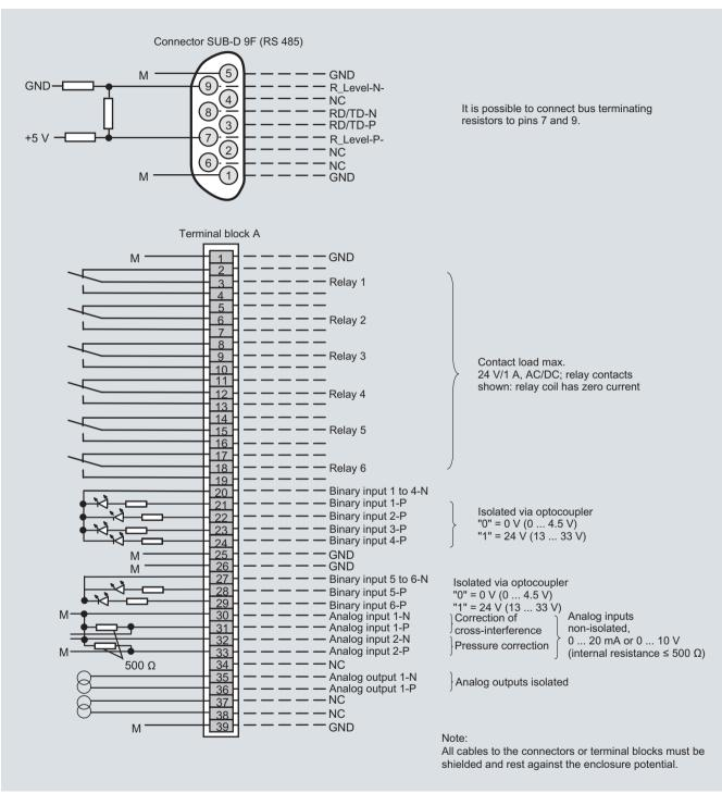
CALOMAT 62, field device, pin and terminal assignment
