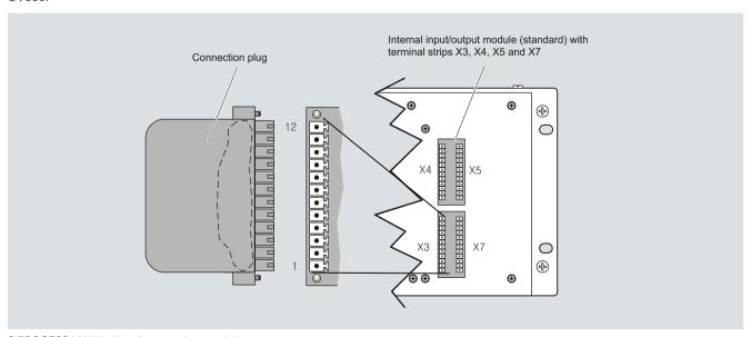
SIPROCESS UV600, signal connections and plug connectors
