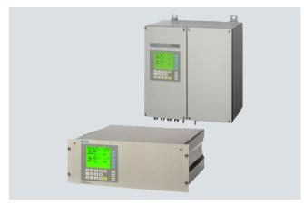
The ULTRAMAT 6 single-channel or dual-channel gas analyzers operate according to the NDIR two-beam alternating light principle and measure gases highly selectively whose absorption bands lie in the infrared wavelength range from 2 to 9  $\mu m$ , such as CO, CO<sub>2</sub>, NO, SO<sub>2</sub>, NH<sub>3</sub>, H<sub>2</sub>O as well as CH<sub>4</sub> and other hydrocarbons.
