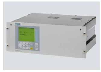
The measuring principle of the OXYMAT 61 gas analyzers is based on the paramagnetic alternating pressure method and is used to measure oxygen in gases in standard applications.
