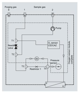
Low-pressure version with integral sample gas pump
