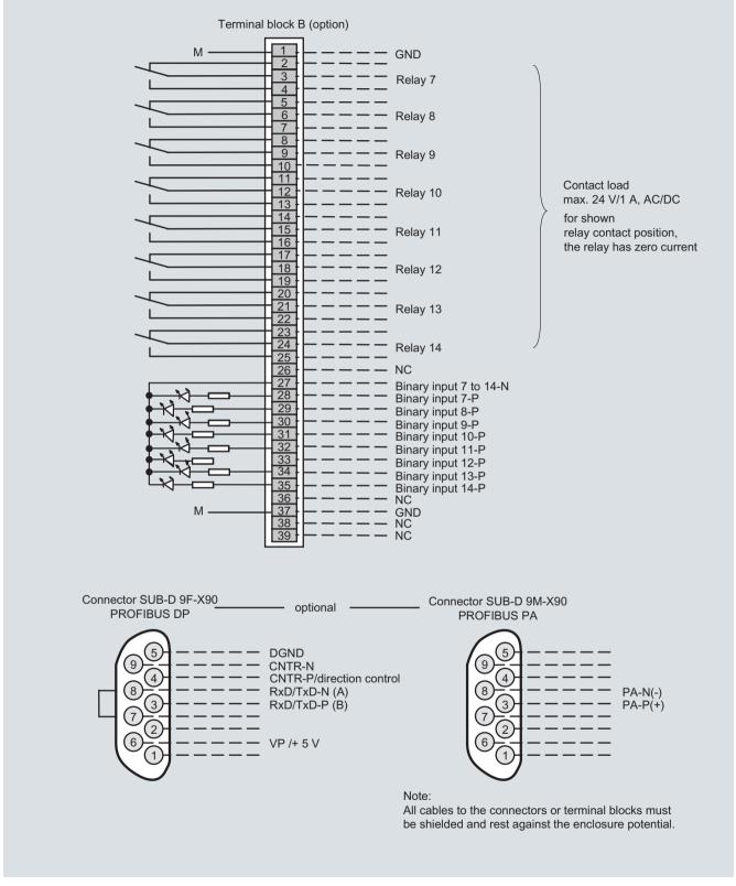
OXYMAT 6, field unit, connector and terminal assignment of the AUTOCAL board and PROFIBUS connectors
