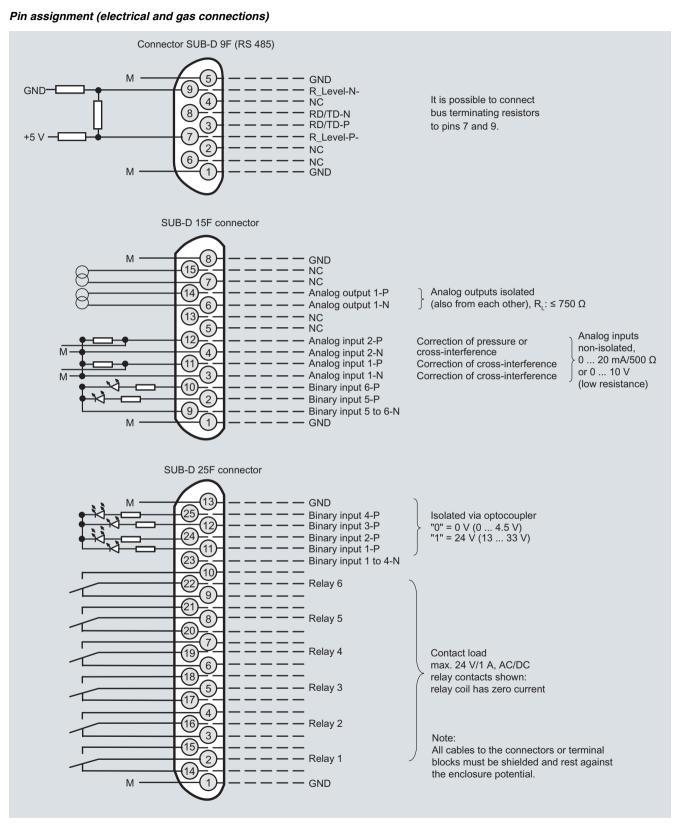
FIDAMAT 6, 19" rack unit, pin assignment
