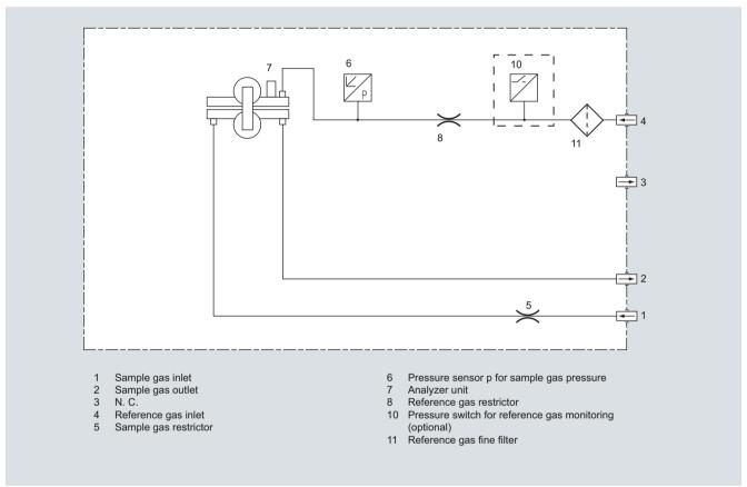
Gas path plan, high-pressure version with optional pressure switch for monitoring reference gas pressure
