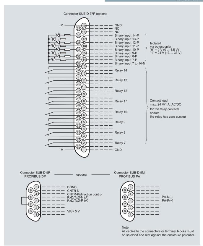
FIDAMAT 6, 19" rack unit, pin assignment of the AUTOCAL board and PROFIBUS connectors
