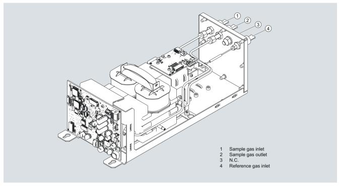
Structure of high-pressure version, sample gas path with pipes
