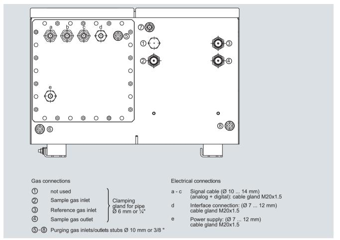
OXYMAT 6, field unit, gas and electrical connections
