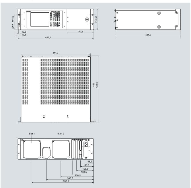
SIPROCESS GA700, rack unit, dimensions in mm
