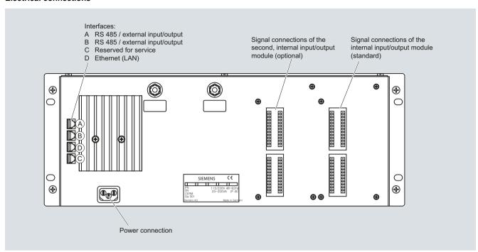
SIPROCESS UV600, gas connections and electrical connections
