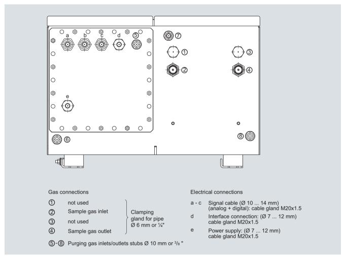
CALOMAT 6, field unit, gas and electrical connections
