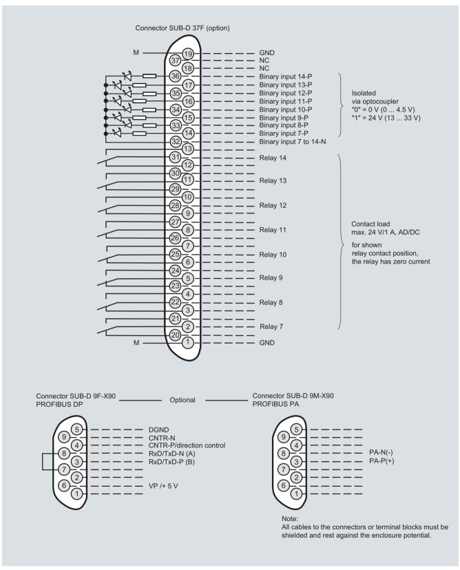
OXYMAT 61, 19" unit, pin assignment of the AUTOCAL board and PROFIBUS connectors
