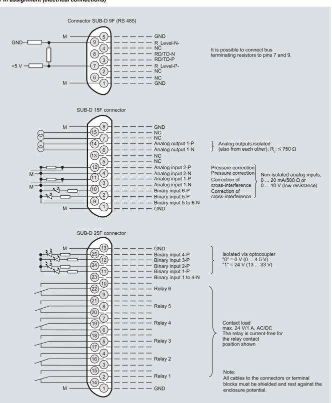
OXYMAT 64, 19" rack unit, pin assignment
