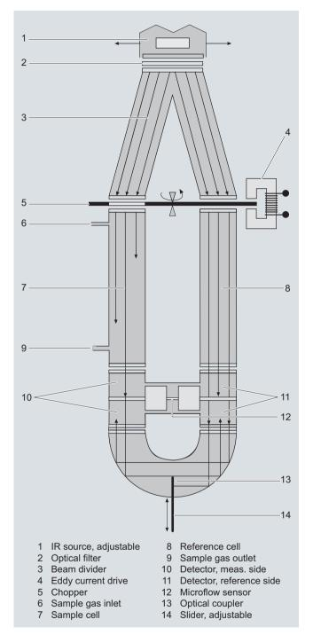
ULTRAMAT channel, principle of operation
