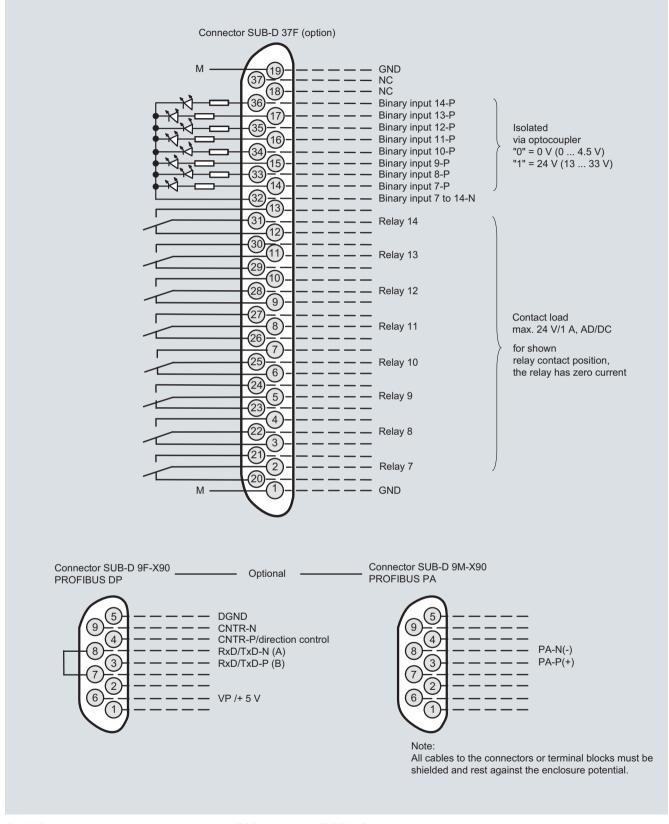
OXYMAT 64, 19" rack unit, pin assignment of the AUTOCAL plate and PROFIBUS plug
