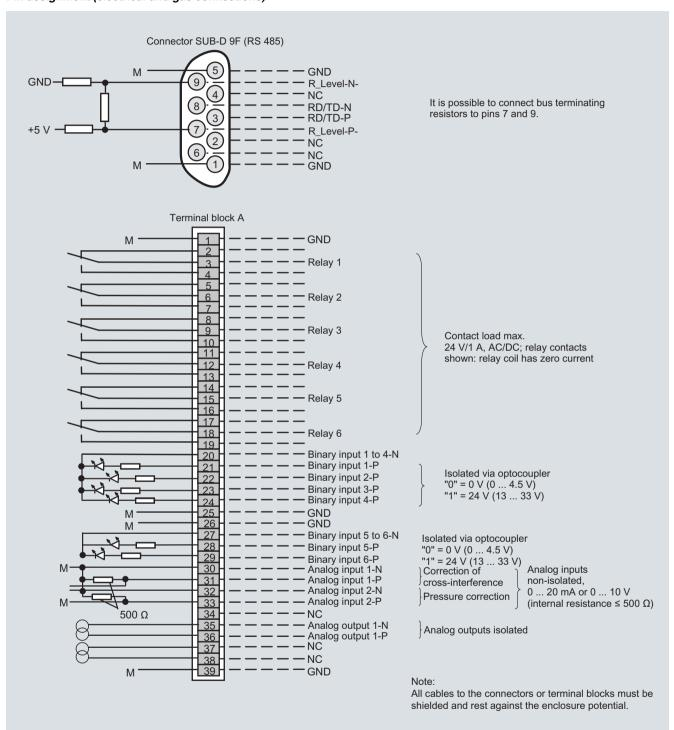
CALOMAT 6, field unit, connector and terminal assignment
