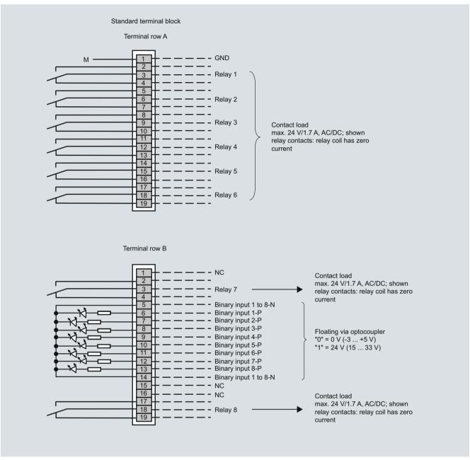
Terminal assignment, standard terminal block, terminal rows A and B
