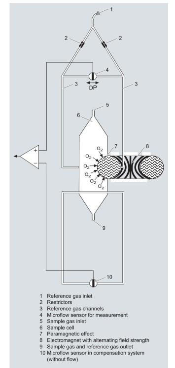
OXYMAT channel, principle of operation
