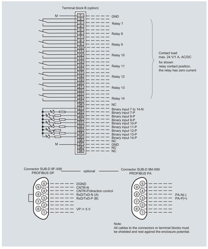
CALOMAT 6, field unit, connector and terminal assignment of the AUTOCAL board and PROFIBUS connectors
