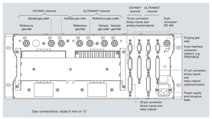
ULTRAMAT/OXYMAT 6, 19" unit, gas and electrical connections
