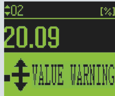
Local user interface (LUI) of SITRANS SL in the detector unit (display of measured value)
