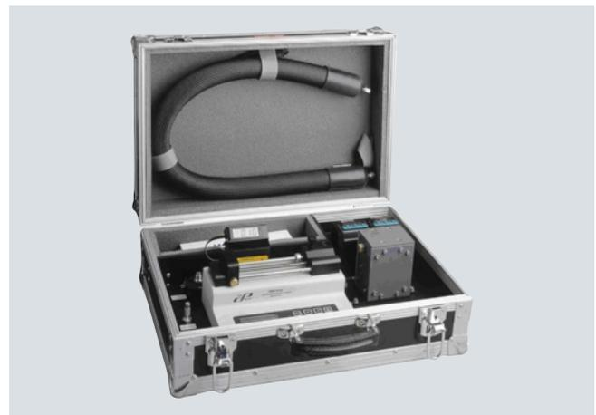
The Gasmet CEMS calibration unit for water
