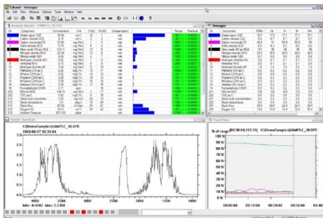
Operator interface of the Calcmet software of the Gasmet CEMS analysis system
