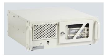
An industrial PC with Windows operating system and RAID hard drives is used in the Gasmet CEMS analysis system for controlling the sampling unit and the analyzers, as well as for data analysis and forwarding of the analysis data to the process control system. The GASMET Calcmet software is used as the control and analysis software.
