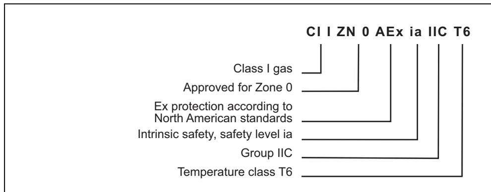
Fig. 9 Example: US identification according to NEC 505
