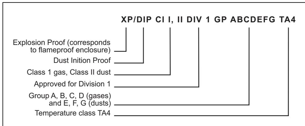
Fig. 8 Example: US identification according to NEC 500
