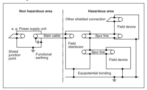
Fig. 15 PROFIBUS PA earthing
