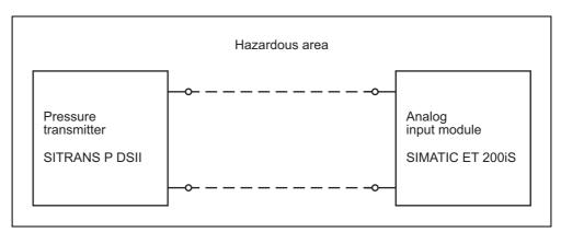
Fig. 12 Connection of a pressure transmitter to an analog input module
