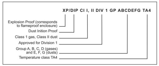
Fig. 8 Example: US identification according to NEC 500
