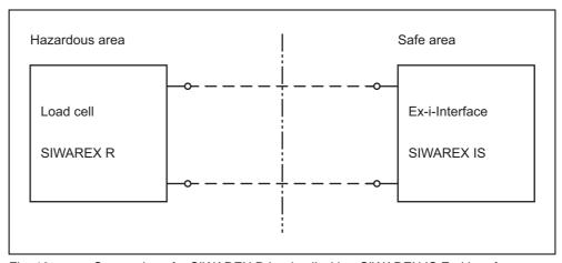
Fig. 13 Connection of a SIWAREX R load cell with a SIWAREX IS Ex-i interface
