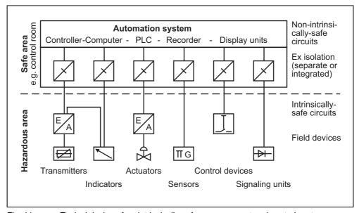
Fig. 11 Typical design of an intrinsically-safe measurement and control system
