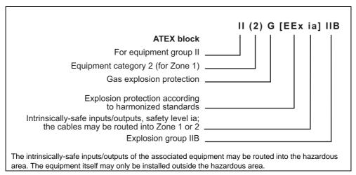
Fig. 7 Example: associated equipment
