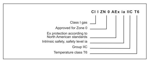
Fig. 9 Example: US identification according to NEC 505
