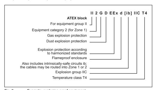
Fig. 6 Example: explosion-proof equipment
