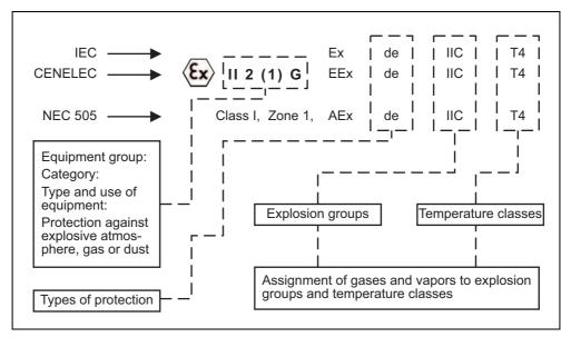
Fig. 4 Identification according to IEC / CENELEC / NEC 505
