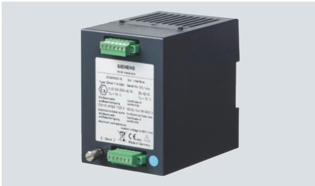
The Ex interface, type SIWAREX IS, can be used for the SIWAREX U, CS, MS, FTA, FTC and CF weighing modules. It contains 6 safety barriers and is labeled according to ATEX and EN 5001U 2D/ II(2)G[EEEx ib] IIC. The Ex interface must be installed outside the potentially explosive area. It should be accommodated in the switchgear cabinet, preferably underneath the weighing electronics, and is secured using a 35-mm rail to EN 50 022.
