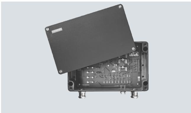
The Ex interface, type SIWAREX Pi, can be used for the SIWAREX U, CS, MS, FTA and FTC weighing modules. It contains 6 safety barriers and has FM approval for devices of Class I Div. 1. The Ex interface must be installed outside the potentially explosive area.
