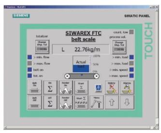
Scale faceplate of a conveyor scale
