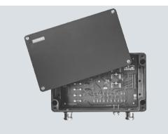
The Ex interface, type SIWAREX Pi, can be used for the SIWAREX U, CS, MS, FTA and FTC weighing modules. It contains 6 safety barriers and has FM approval for devices of Class I Div.1. The Ex interface must be installed outside the potentially explosive area.
