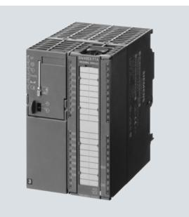
The SIWAREX FTA (Flexible Technology, Automatic Weighing Instrument) is a versatile and flexible weighing module designed for industrial use. It can be used for both automatic and non-automatic weighing, e.g. for the production of mixtures, or for filling, loading, monitoring or bagging.
