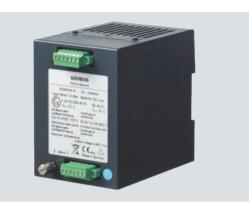
The Ex interface, type SIWAREX IS, can be used for the SIWAREX U, CS, MS, FTA, FTC and CF weighing modules. It contains 6 safety barriers and is labeled according to ATEX and EN 5001U 2D/ II(2)G[EEx ib] IIC. The Ex interface must be installed outside the potentially explosive area. It should be accommodated in the switchgear cabinet, preferably underneath the weighing electronics, and is secured using a 35-mm rail to EN 50 022.
