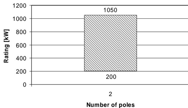
Power range of 1PQ8 High-Speed motors (dependent on the number of poles) for:
