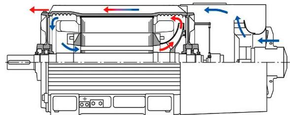
*Cross-section of a 1PQ8 motor*
