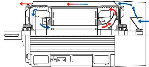
*Cross-section of a 1LA8 Standardline motor*
