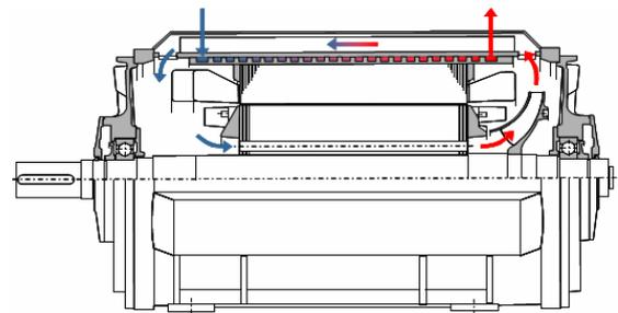
*Cross-section of a 1LH8 motor*
