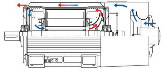
*Cross-section of a 1PQ8 motor*
