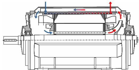
*Cross-section of a 1LH8 motor*
