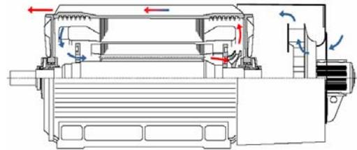
*Cross-section of a 1PQ8 High-Speed motor*
