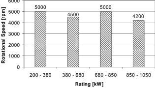
Rotational speed range of 1PQ8 High-Speed motors (dependent on the power)
