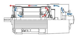
Cross-section of a 1PQ8 motor
