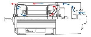
Cross-section of a 1PQ8 motor
