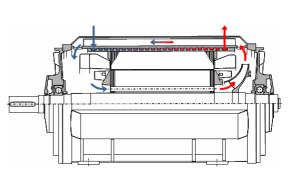
Cross-section of a 1LH8 motor
