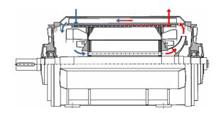
Cross-section of a 1LH8 motor
