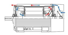
Cross-section of a 1LA8 Standardline motor
