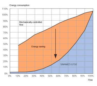
Comparison of energy consumption with mechanicallycontrolled and converter-controlled flow
