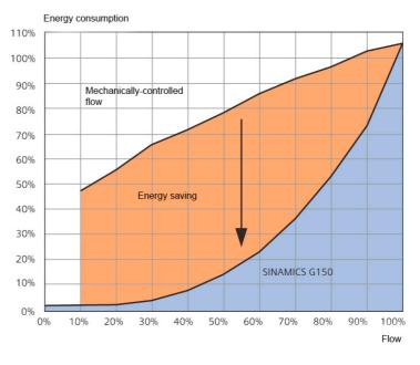
Comparison of energy consumption with mechanicallycontrolled and converter-controlled flow
