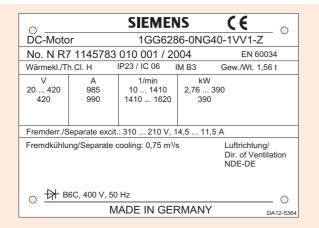
Rating plate for motors of frame sizes 160 to 630
