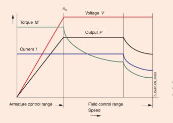
$n_N$ Rated speed Max. field weakening speed at  $P_{\rm N}$  = constant n<sub>Fmax</sub> Max. permissible operating speed n<sub>mech</sub>
