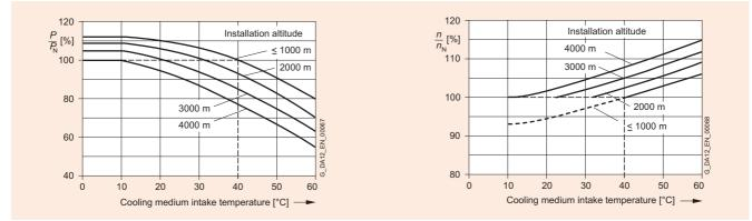
Output (left) and speed deviations (right) as a function of installation altitude and the cooling medium intake temperature
