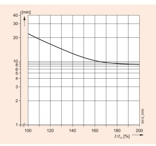
Thermal equivalent time constant  $T_{\text{therm}}$
