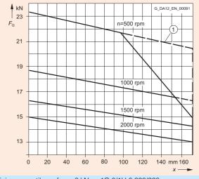
Minimum cantilever force 6 kN 1G.6/1H.6 226/228
