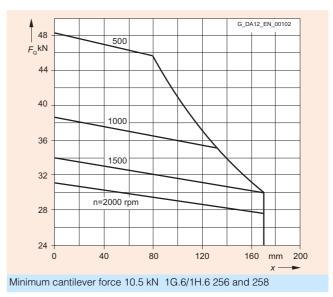
Motors 1G.6/1H.6 with special design bearings for extremely high cantilever forces are longer.
