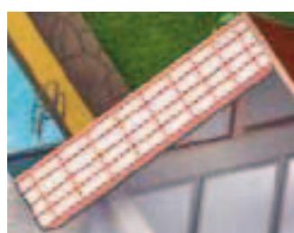
**12** - The roof temperature can be monitored instant by instant by means of the **THS**, so as to turn on the heating elements and prevent ice from forming.
