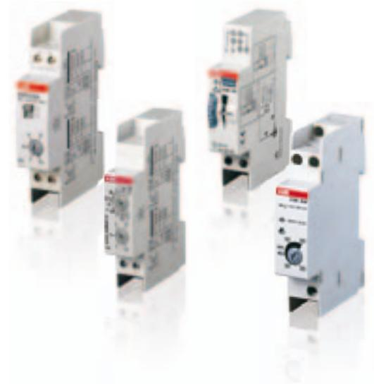
E 232E-8/230 devices feature an additional, separate control input with an universal voltage of 8 to 230 V AC/DC. The "Multi 10" versions also feature the integrated alarm function (2 flashing alarm signals) in accordance with DIN 18015-2 standards and a rotary selector on the front with 10 functions to choose from, divided into 4 types: timed relay mode, latching relay mode, timed latching relay mode and permanently on mode.
