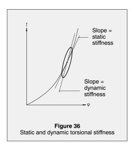
For couplings the dynamic stiffness is given, as a rule, which is measured at a vibrational
