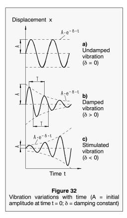
If the vibrating system is excited by a periodic external force F(t) or moment M(t), this is a forced or stimulated vibration. With the periodic external excitation force, energy can be supplied to or removed from the vibrating system.
