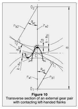
In a cylindrical gear pair either the left or the right flanks of the teeth contact each other on the line of action. Changing the flanks results in a line of action each lying symmetrical in relation to the centre line through  $O_1$   $O_2$ . The line of action with contacting left flanks in figure 10 is the tangent to the two base circles at points  $T_1$  and  $T_2$ . With the common tangent on the pitch circles it includes the working pressure angle  $\alpha_{\text{Wt}}$ .
