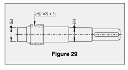
Datum system formed by two datums (directional datum "A" and short axis "B").
