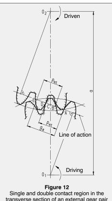
transverse section of an external gear pair
