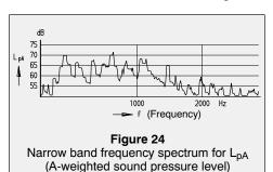
Histograms occur in the one-third octave spectrum and in the octave spectrum, see figures 25 and 26. In the one-third octave spectrum (spectrum with 1/3 octaves), the bandwidth results from
