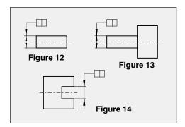
on the axis or the median plane when the tolerance refers to the common axis or median plane of two or more features (see figure 15).
