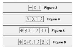
Remarks referred to the tolerance, for example "6 holes", "4 surfaces", or "6 x" shall be written above the frame (see figures 7 and 8).
