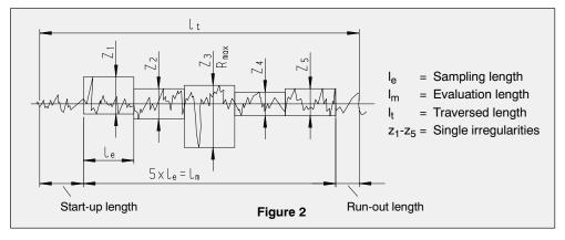
An exact conversion of the peak-to-valley height Rz into the centre line average height Ra and vice versa can neither be theoretically justified nor empirically proved. For surfaces which are generated by manufacturing methods of the group "metal cutting", a diagram for the conversion from Ra into Rz and vice versa is shown in supplement 1 to DIN 4768, based on comparison measurements. The Ra values assigned to the Rz values are subject to scattering (see table).
