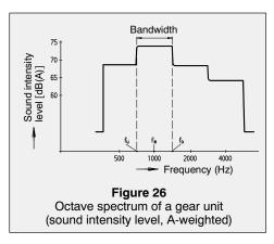
The total level (resulting from logarithmic addition of individual levels of the recorded frequency range) is a single-number rating. The total level is the common logical value for gear unit noises. The sound pressure level is valid for a certain distance, in general 1 m from the housing surface as an ideal parallelepiped.
