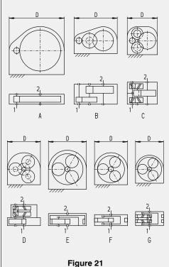
Diagrammatic view of cylindrical gear unit types without and with load sharing. Transmission ratio i = 7. Size comparison to scale of gear units with the same output torque.
