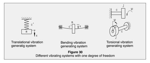
Further, a distinction is made between free vibrations and externally forced vibrations, and whether the vibration takes place without energy losses (undamped) or with energy losses (damped).
