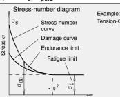
In case of stresses below the damage curve initial damage will not occur to
