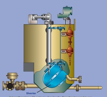
Veirsep™ system with cutaway showing the flow diverter used to concentrate the flow in the path of bubbles as well as the manipulation of surface tension to force the float towards the adjustable weir.
