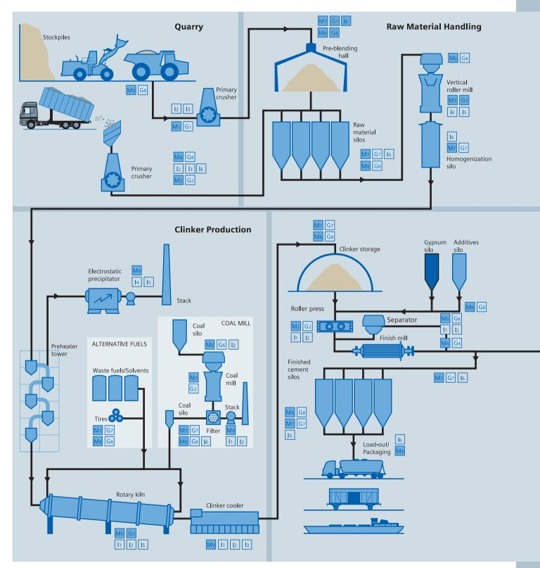
From quarry to kiln, from clinker silo to loading – the entire process chain of a cement plant with daily clinker production of up to 12,500 tonnes requires supreme performance and efficiency. The drive technology used not only has to handle continuous operation, sometimes for over 300 days a year, but must also withstand the toughest environmental conditions. Siemens/Flender offers bespoke and highly reliable drive systems
