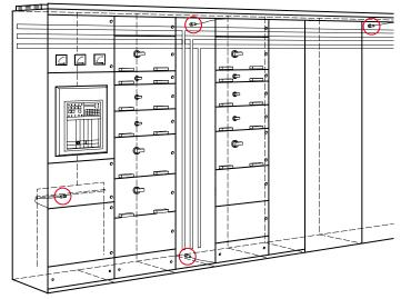
Example showing the position of detectors in: 1. Horizontal and vertical bus bar system
