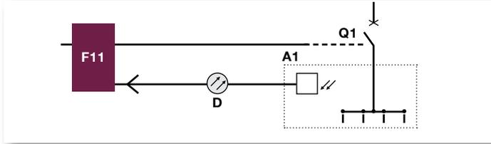
F11 Arc Monitor, Q1 Circuit breaker, A1 Switchgear, D Detector
